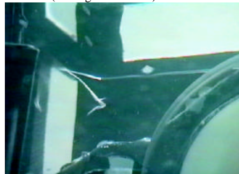
Fig.11 Diffuser inlet, opposite fan cut-off wall, (8 volts, 1200 rpm).
